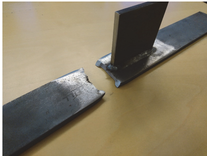
Figure 5: One of the six specimens tested, showing the fracture in the predicted location for this class of welded joints. All the specimens showed the same kind of failure.
