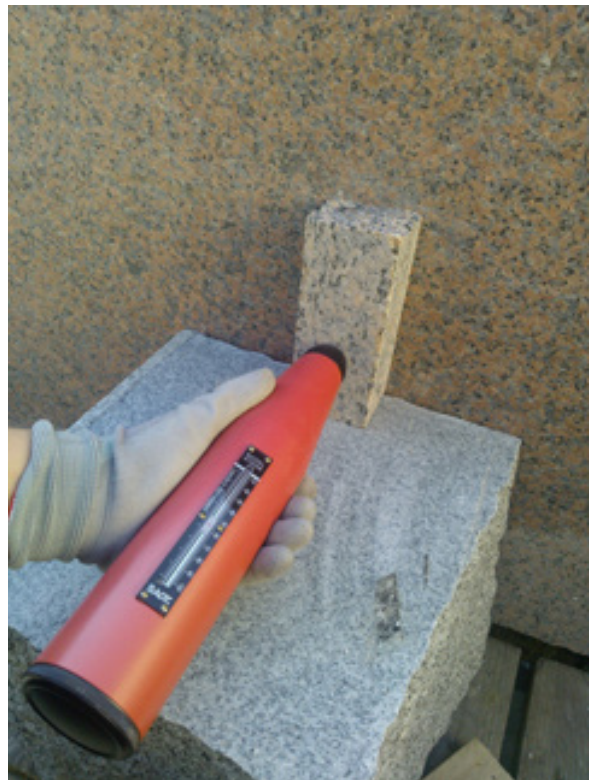
Figure 5. Schmidt rebound hammer instrument in testing position. Photo: Nike Luodes.
