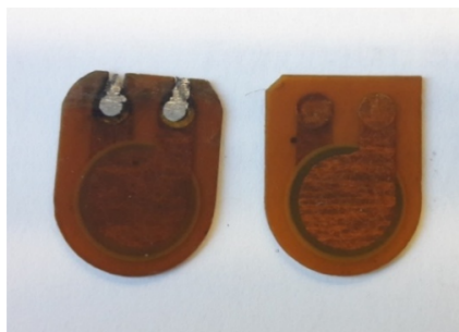
Figure 4: Wide-band ceramic PZT “DuraAct” kapton encapsulated.
