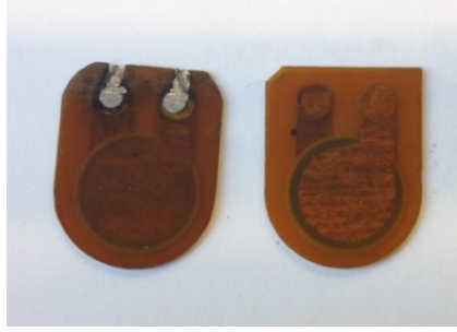
Figure 4: Wide-band ceramic PZT “DuraAct” kapton encapsulated.
