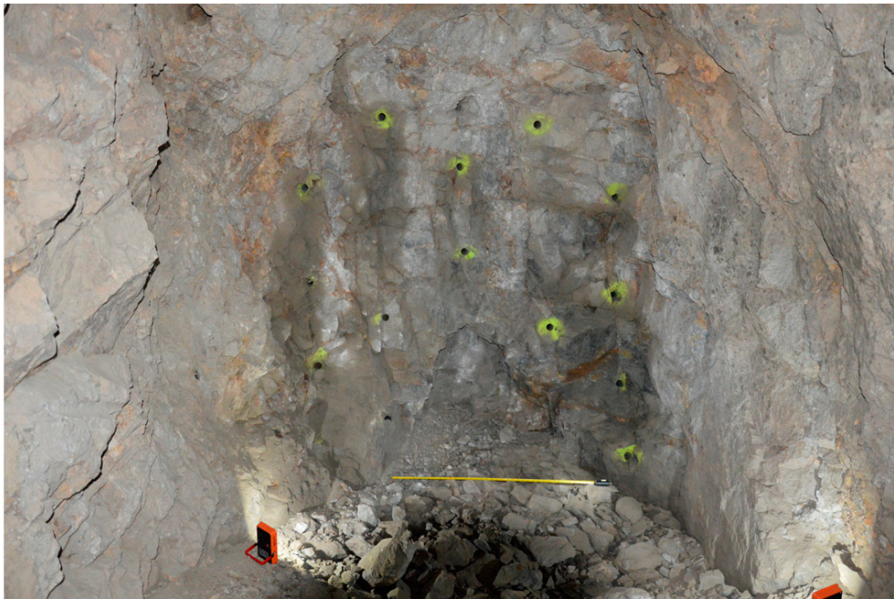
Figure A7. Cavity after detonation of hole with sequence number 6.
