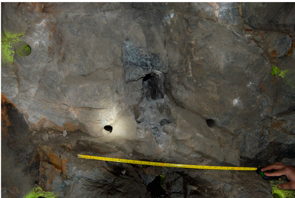
Figure A2. Cavity after detonation of hole with sequence number 1.
