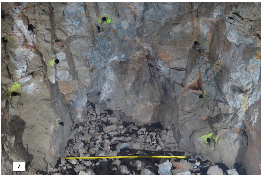
Figure A8. Cavity after detonation of hole with sequence number 7.
