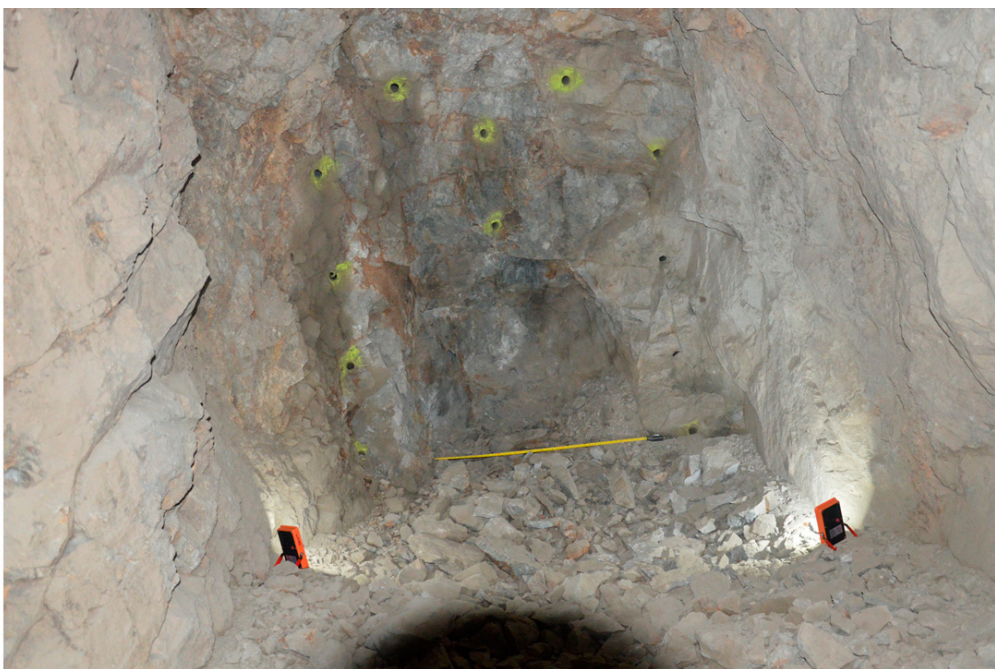
Figure A10. Cavity after detonation of hole with sequence number 9.
