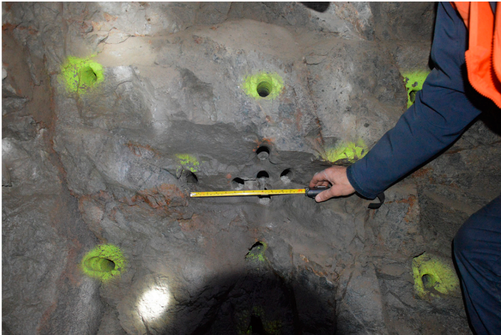
Figure A1. Burn cut after detonation of central hole with sequence number zero.
