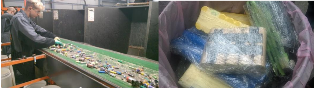
Figure 53: Sorting of batteries at the Van Peperzeel plant (The Netherlands)
