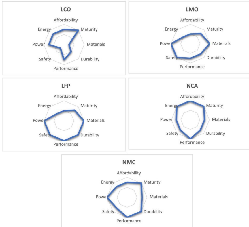
Figure 40. Main characteristics of Li-ion batteries (Zubi et al., 2018)
