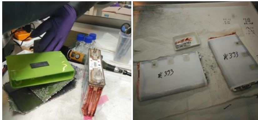
Figure 50: Dismantling of the Mitsubishi Outlander PHEV battery pack
