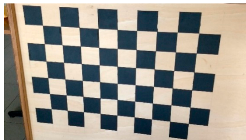
Figure 3. Wooden panel with checkerboards for the camera calibration. Each box measures 10 cm.
