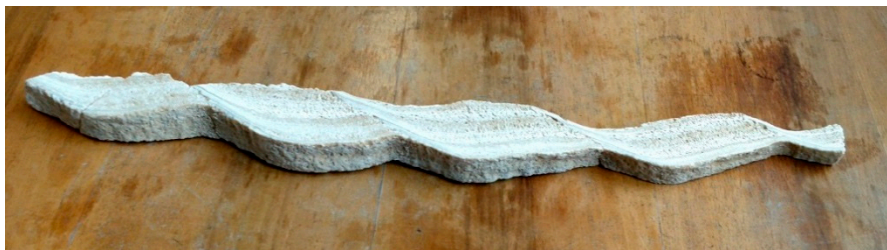
Figure 1. The calcareous rock sample used for the test.
