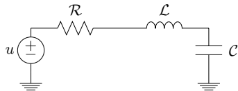
Fig. 11. The RLC electrical circuit considered in Example 5.
