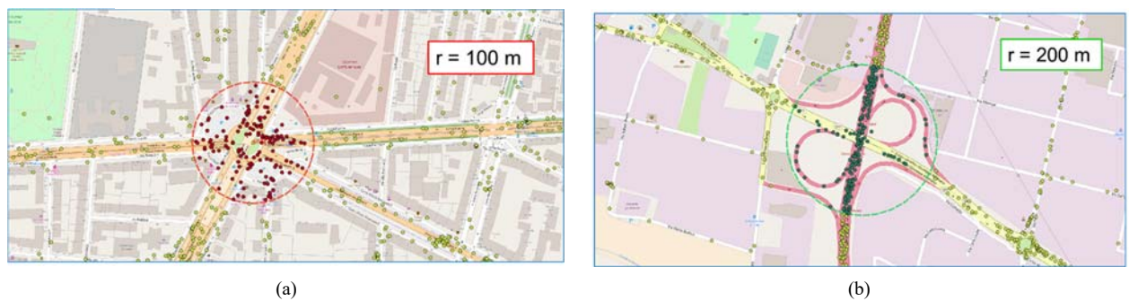
Figure 2 Two examples of different diameter options for the matching between nodes and positioning data: a two lanes road (a) and a motorway case (b).
