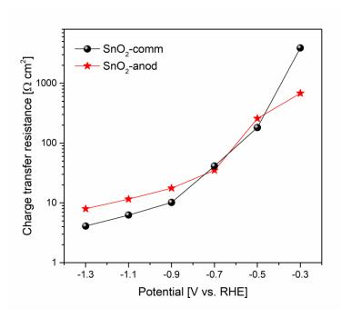
Figure S12 Comparison of charge transfer resistance obtained from EIS on SnO<sub>2</sub>-comm and SnO<sub>2</sub>-anod electrodes at various potentials.
