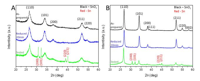
Figure S4 XRD patterns of (a) SnO<sub>2</sub>-anod and (b) SnO<sub>2</sub>-comm electrodes (as-prepared, reduced for 20min and tested).
