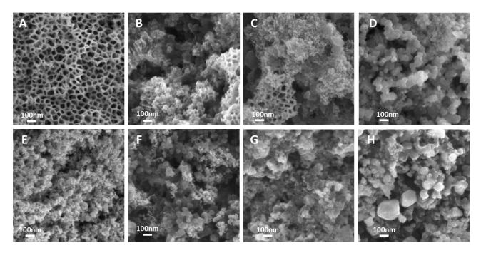
Figure S1 Top view FESEM images of the (a) as-grown SnO<sub>2</sub>,(b) as-prepared electrode SnO<sub>2</sub>-anod, (c) SnO<sub>2</sub>-anod electrode reduced for 20min and (d) tested SnO<sub>2</sub>-anod electrode, (e) commercial SnO<sub>2</sub>, (f) as-prepared electrode SnO<sub>2</sub>-comm, (g) SnO<sub>2</sub>-comm electrode reduced for 20min and (h) tested SnO<sub>2</sub>-comm electrode. All images are shown at the same magnification.
