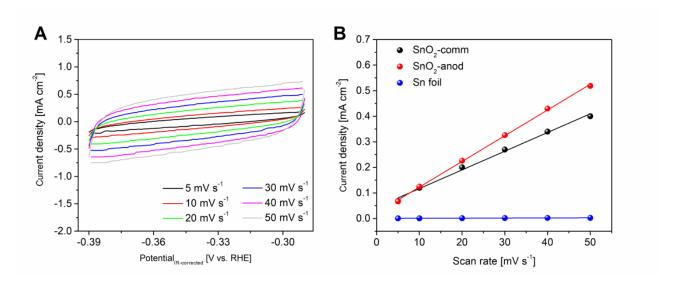
Figure S7 Determination of double-layer capacitance for various electrodes in CO<sub>2</sub>-saturated 0.1 M KHCO3: (a) representing CVs on SnO<sub>2</sub>-anod electrode; (b) Capacitance values calculated from the slopes of current densities vs. scan rate.
