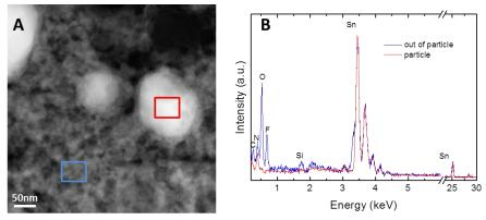
Figure S15 STEM image of the cross-section lamella of tested SnO<sub>2</sub>-anod electrode (a) and EDX measurement performed locally in the particle and out of the particle (b).
