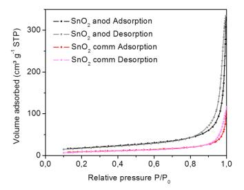
Figure S2 N<sub>2</sub> adsorption/desorption isotherms for SnO<sub>2</sub> prepared via anodic oxidation and commercial.
