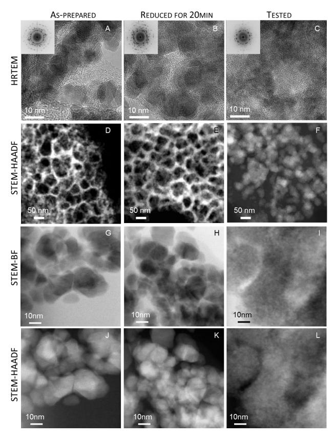
Figure S6 TEM study of the crystals evolution of the SnO<sub>2</sub>-anod, including the as-prepared, reduced for 20 minutes and long term tested material. In the rows the following images are shown: HRTEM with FFT (of the shown area) in the inset, low magnification HAADF-STEM image, high magnification BF-STEM and HAADF-STEM.
