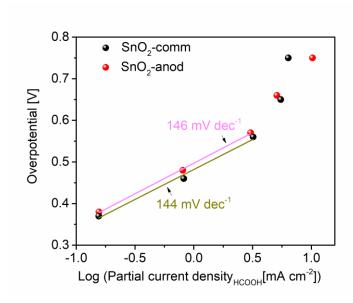
Figure S13 Tafel plot analysis for HCOOH production on SnO<sub>2</sub>-comm and SnO<sub>2</sub>-anod electrodes.
