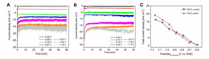
Figure S11 CA measurements carried out in CO<sub>2</sub>-saturated 0.1 M KHCO<sub>3</sub> aqueous solution at different potentials: (a) SnO<sub>2</sub>-comm; (b) SnO<sub>2</sub>-anod; (c) Comparison of total current densities on SnO<sub>2</sub>-comm and SnO<sub>2</sub>-anod electrodes at various potentials.
