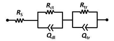
Figure S10 Equivalent circuit used for fitting of EIS data.
