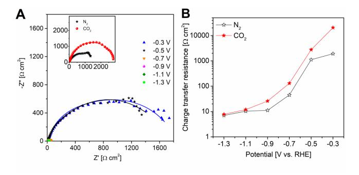
Figure S9 EIS analysis on a Sn foil electrode: (a) Nyquist plots obtained in  $N_2$ -saturated electrolyte (the points are experimental data, the clines are the curves calculated through fitting. In the inset, the two spectra acquired at -0.5 V in  $N_2$ - and  $CO_2$ -saturated solutions are shown. (b) Charge transfer resistances reported as a function of the potential.
