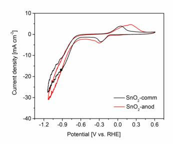
Figure S8 Comparison of the voltammograms of SnO<sub>2</sub>-comm and SnO<sub>2</sub>-anod in the CO<sub>2</sub>-saturated electrolyte.
