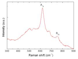
Figure S5 Raman spectrum of as-prepared SnO<sub>2</sub>-anod electrode.
