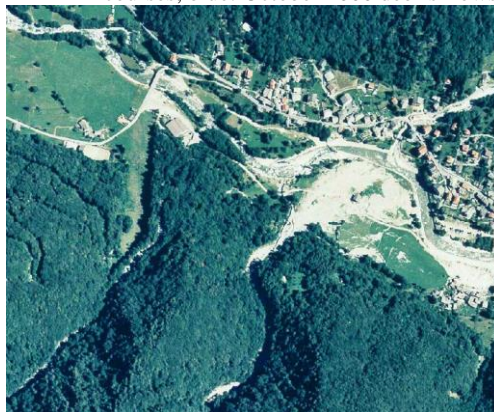
Fig. 2.2 Cuccetta (on the left) and Urtorei (on the right) alluvial fans, after October 2000 debris flows (Flight “Alluvione 2000” Regione Piemonte, 2001)
