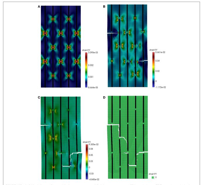
FIGURE 6 | Strain fields during tensile test of the heterogeneous matrix/reinforcement structure. (A) linear elastic part. (B) Tips cracks opening leading to the plastic part. (C) debonding leading to the material failure (D).
