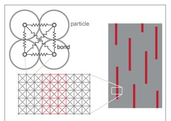
FIGURE 1 | Schematic of the adopted hierarchical lattice spring model (HLSM), illustrating the network of "springs" connecting nodes in which the material is discretized at different size scales. Different mechanical properties assigned to the springs (represented in different colors on the right) correspond to different material portions, e.g., matrix and reinforcements in a composite material (right).
