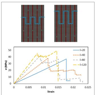
FIGURE 8 | Top: structure of model composites with varying reinforcement aspect ratios (I/w = 40 and I/w = 80), with schematic crack propagation paths. Bottom: corresponding stress-strain curves for varying reinforcement aspect ratios. Increasing aspect ratio leads to increasingly stiff behavior.
