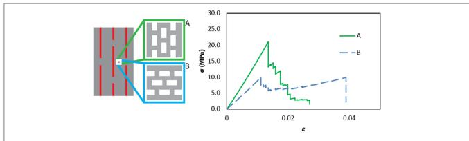
FIGURE 10 | Incorporation of "A" type and "B" type RVEs in the matrix of a reinforced composite in a multi-scale hierarchical scheme. The corresponding stress—strain plots are shown on the right. As expected, "A" type RVEs give rise to a stiffer, stronger composite, while "B" type elements yield a softer, tougher composite.
