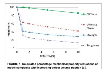
hierarchical level (the "composite" level) are shown in Figure 7 for varying volume fractions of defects in the matrix. The figure illustrates the percentage degradation of stiffness, ultimate strain, strength, and toughness of the resulting composite, normalized
