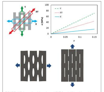
FIGURE 9 | Schematic of the adopted RVE (top left) in a hierarchical multi-scale simulation, and its resulting stress-strain behavior (top right). The element is stiffer and stronger in the longitudinal direction (Y axis) with respect to the transverse direction (X axis), while springs in the diagonal direction (XY) have intermediate properties. The resulting deformation for loading in the X and Y directions is illustrated at the bottom left and right of the figure, respectively.
