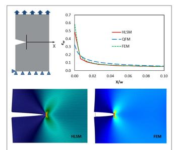
**FIGURE 3 | HLSM simulation results for a tensile loading experiment on a laterally cracked RVE (schematic, top left).** Vertical strain YY results along the *X* axis coincide with those from FEM simulations and quantized fracture mechanics (QFM) calculations, shown in the plot (top right). HLSM and FEM simulations also predict the same full-field strain distributions at the crack tip (bottom left and right, respectively).
