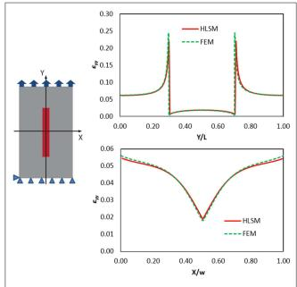
**FIGURE 4 | HLSM simulation results for a tensile loading experiment on a centrally reinforced RVE (schematic on the left).** Strain YY variation along *X* and *Y* axes normalized with respect to width w and length L (bottom right and top right, respectively) compared to that of FEM simulations.
