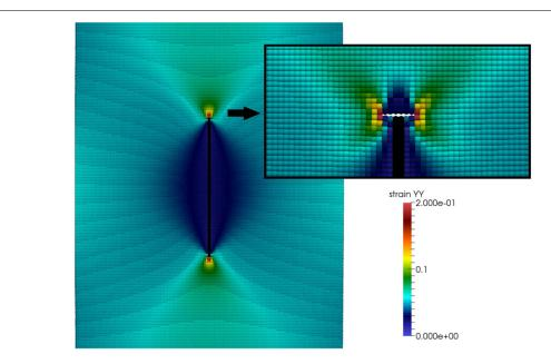
FIGURE 5 | YY Strain field calculated using HLSM model for a vertically loaded RVE with a centrally embedded stiff linear elastic inclusion. The inset highlights the strain concentration at the tips of the reinforcement, giving rise to crack nucleation and propagation.
