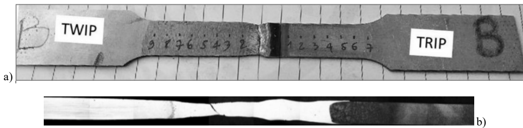
Fig. 15. a) Macro-specimens after a tensile test run; b) Etched cross-section of a fractured macro-sample. Nital etching used for image b).
