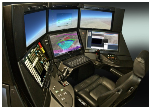
Figure 3 – Example of RPAS Ground Control Station [7]
