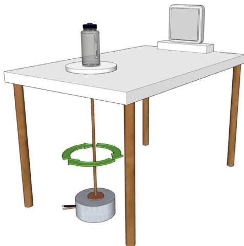
Fig. 1. a) Sketch of the test bench and b) picture of the UH 105 Lab-ID transponder attached on the empty flask.
