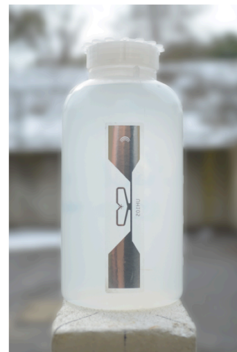
Fig. 1. a) Sketch of the test bench and b) picture of the UH 105 Lab-ID transponder attached on the empty flask.
