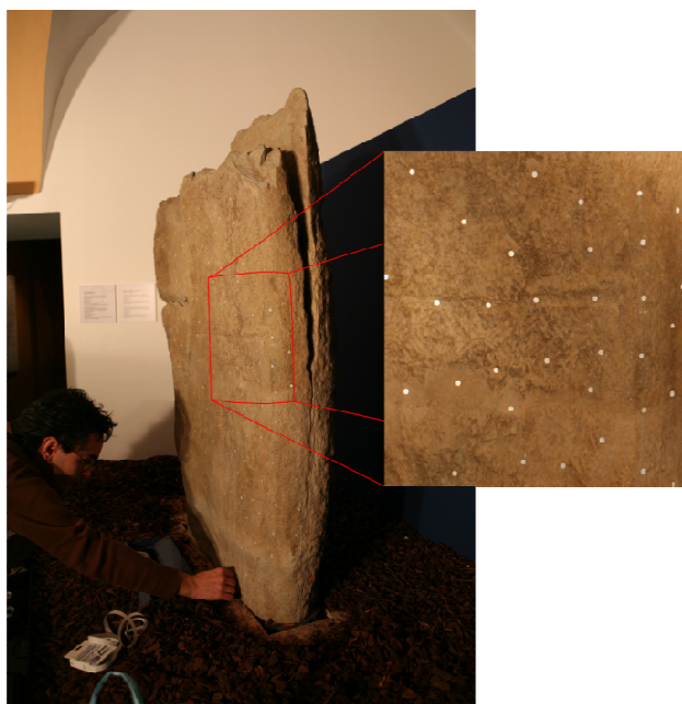
Figure 5. Placing the reflective targets on the object
