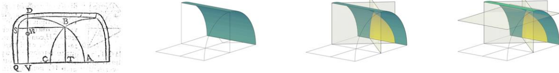
Fig. 12. Guarini, surface to be subtracted for inserting a lunette. (Source: Guarini, 1674, Proposition 16. Modelling: author).
