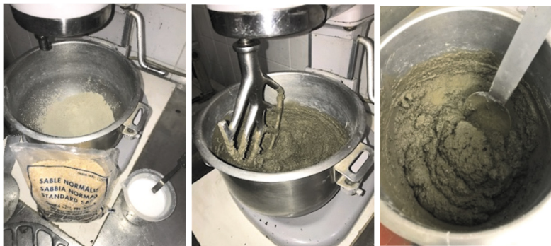
Figure 2. Preparation cement mortar mixtures
