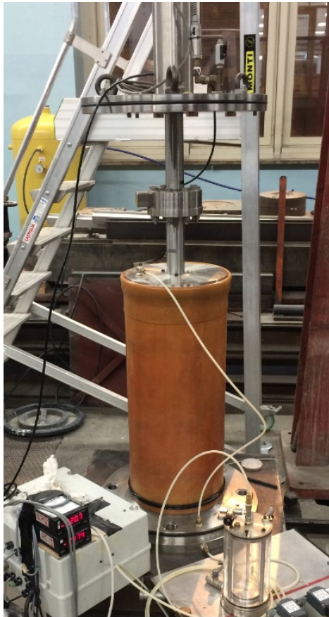
Figure 4: Dry sand sample with the external depression applied
