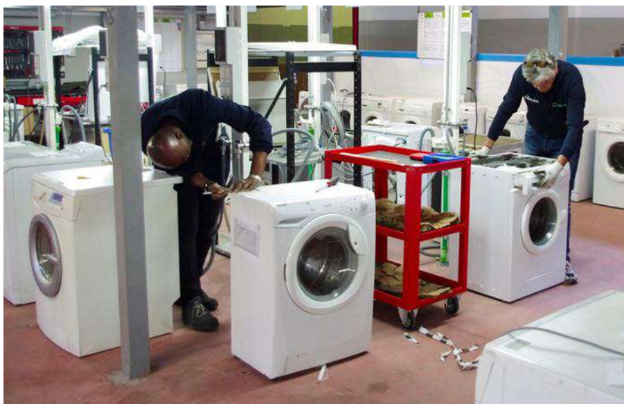
Figure 3. Check and regeneration of the appliances in the Ri-Generation laboratory (credits: Ri-Generation).
