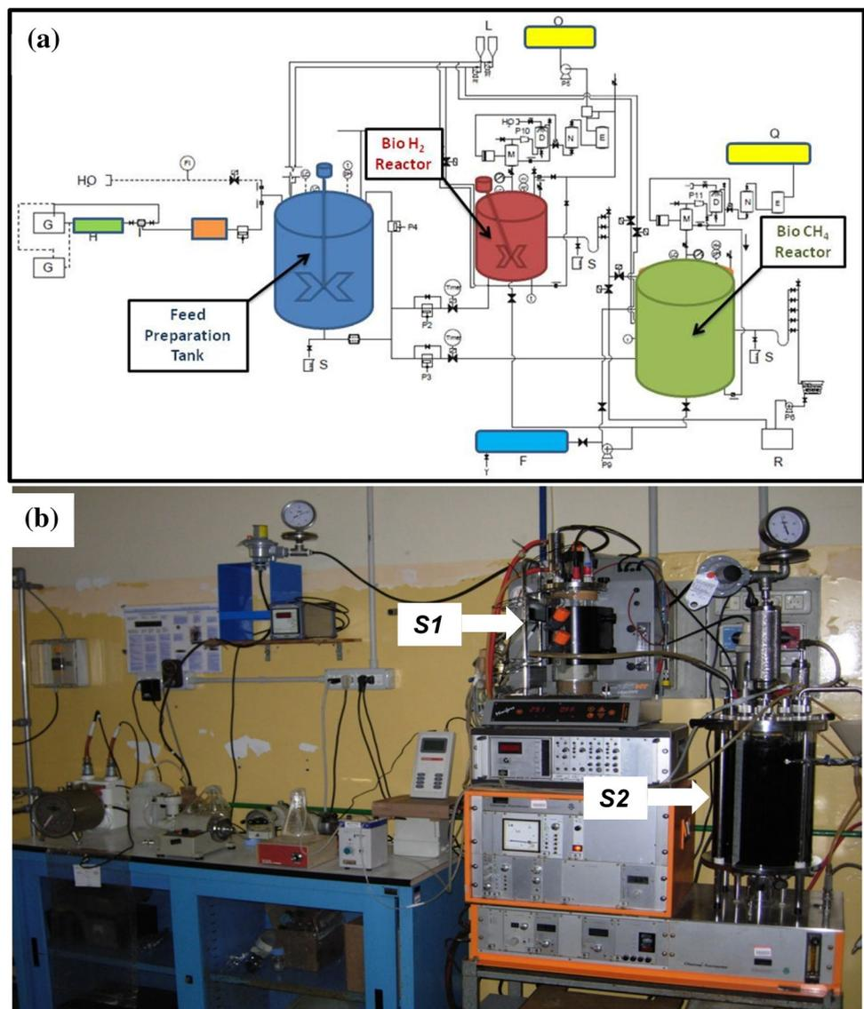
unnecessary water expenditure and to satisfy the water content requirements for the DF process for wet fermentation. However, in the case of TSAD, the water recycling stream also contains some HCB concentrations, which should not introduce any significant perturbations to the microbial composition in S1. In this respect, the output stream of S2 is filtered using 125 µm nylon filters (Carl Roth GmbH, Karlsruhe, Germany) and used to dilute the feed for S1.
