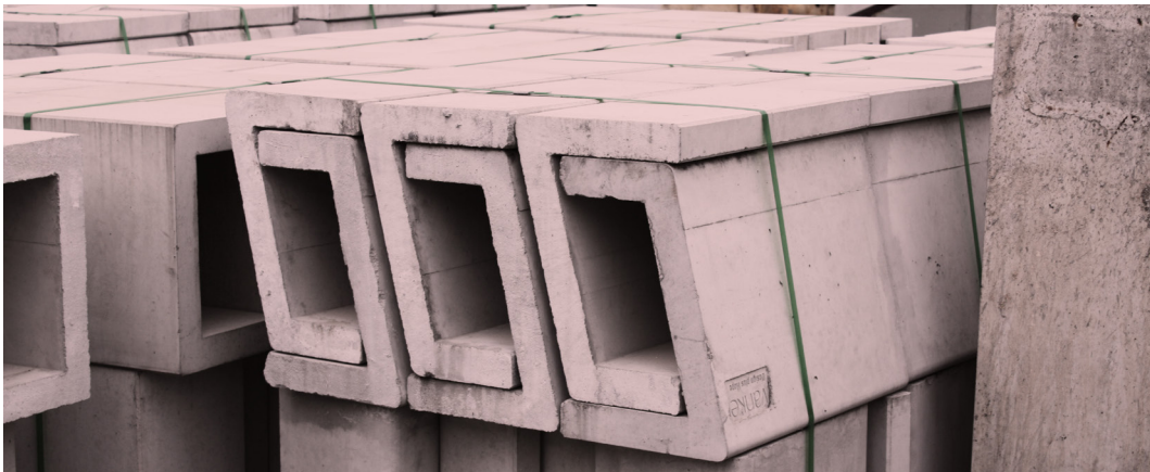
Figure 7.53: Pre-cast concrete landscape elements in Vanke's Housing Industrialization Research Center in Dongguan (source: picture by the author).
