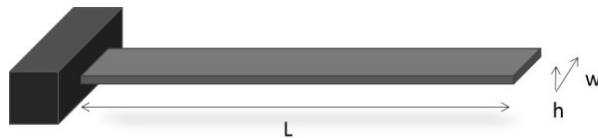
Figure 2.1 Graphical representation of a single clamped beam (cantilever).
