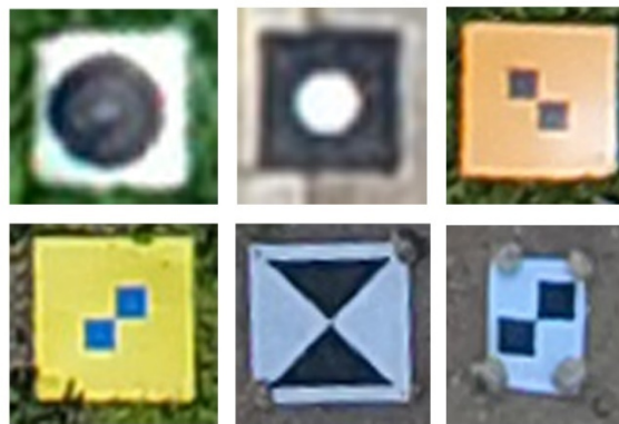
Figure 1 Some examples of different typologies of codified targets
