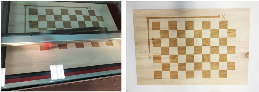
Figure 100 The wooden checkboard panel used for the calibration procedure. On the left the CNC machine during the cutting phase
