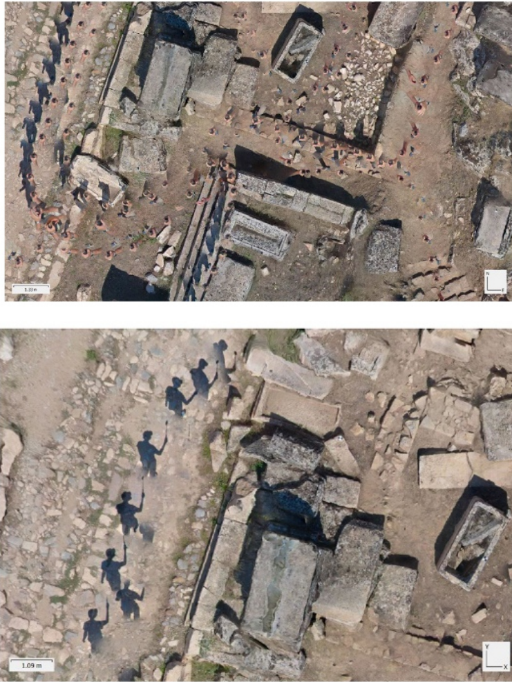
Figure 150 Hierapolis, Northern Necropolis. Examples of aberration that can be present on the orthoimage generated from the 360 dataset
