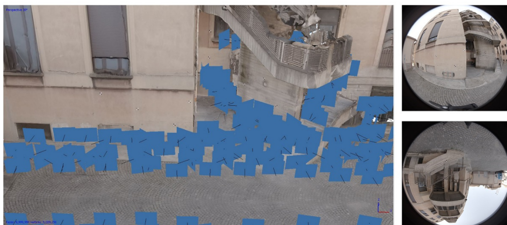
Figure 121 Acquisition scheme of the 3D calibration field achieved with the GoPro Fusion and example of acquired images
