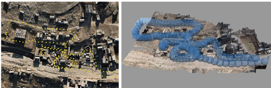
Figure 144 Hierapolis, Northern Necropolis dataset 3. Acquisition scheme of the data collected in time lapse mode with the GoPro Fusion. Camera stations showed on an extract of the UAV's orthophoto (left) and on the 3D model in the photogrammetric software (right)
