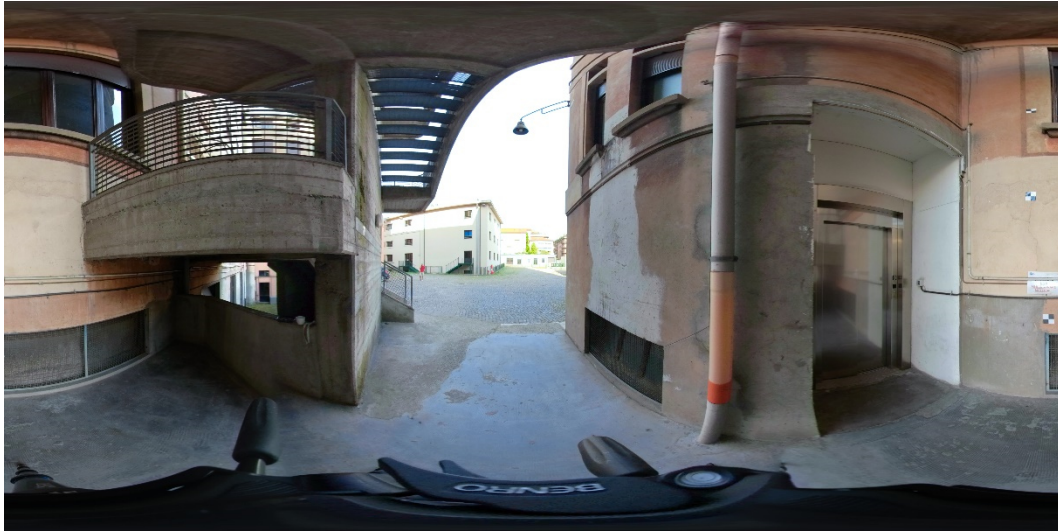
Figure 130 Example of spherical image of the calibration field derived from the stitching of front and back camera of GoPro Fusion
