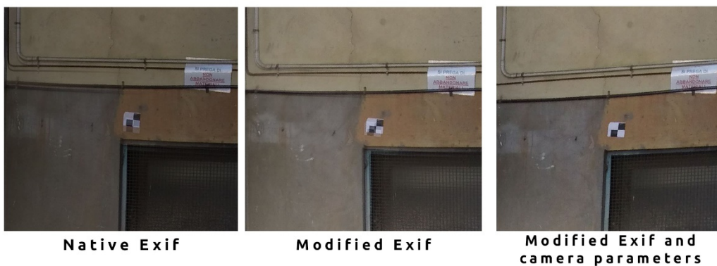
Figure 117 Stitching aberration related with the use of different approach for camera interior parameters estimation
