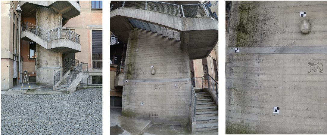
Figure 102 The calibration field and a detail of some of the target distributed on its surface
