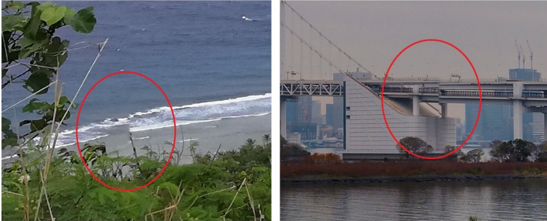
Figure 41 Examples of ghosting (left) and parallax (right) errors in the stitching process.
