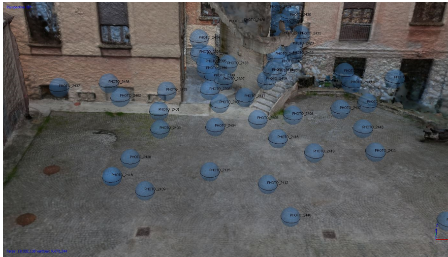
Figure 131 View of the acquisition scheme achieved with the GoPro Fusion
