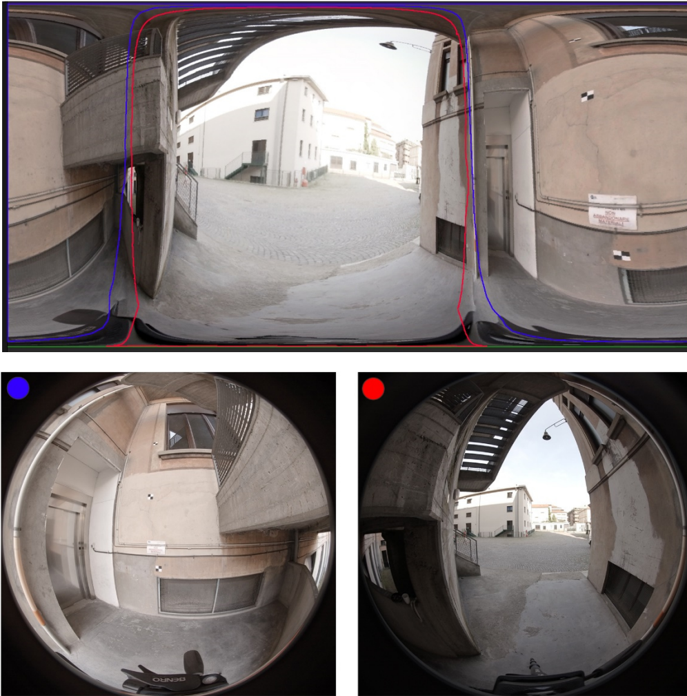
Figure 129 GoPro Fusion. Stitching of the two cameras and overlapping areas between images
