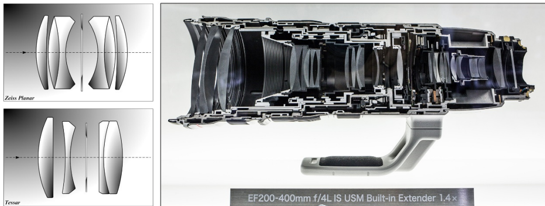
Figure 22 Examples of symmetrical lens design (Zeiss Planar on the top left) and asymmetrical lens design (Tessar's design on the down left). On the right part of the images a section of a Canon lens. 15
