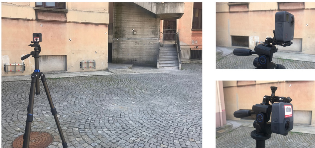
Figure 120 Some phases of acquisition of the 3D calibration field with the GoPro Fusion
