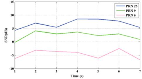
Figure 3. Sky-plot (top). SNR for PRN23, PRN9 and PRN6 (Bottom).
