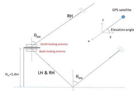
Figure 1. The basic architecture of GNSS-R system.
