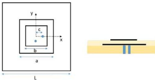
Figure 4. The geometry of the dual CP patch.
