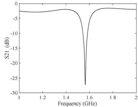
Figure 6. Simulations of the hybrid coupler isolation..
