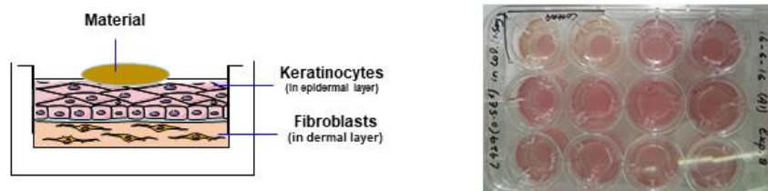
Figure 9.8 Test design - Cytotoxicity testing of H 2 O 2 releasing 10% HB-PEGDA/1% HA-SH hydrogels on in vitro 3D skin model (HSE).
