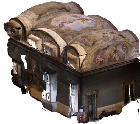
Figure 8. Textured mesh model from PhotoScan - 'Prima Anticamera' (Modelling: F. Natta)
