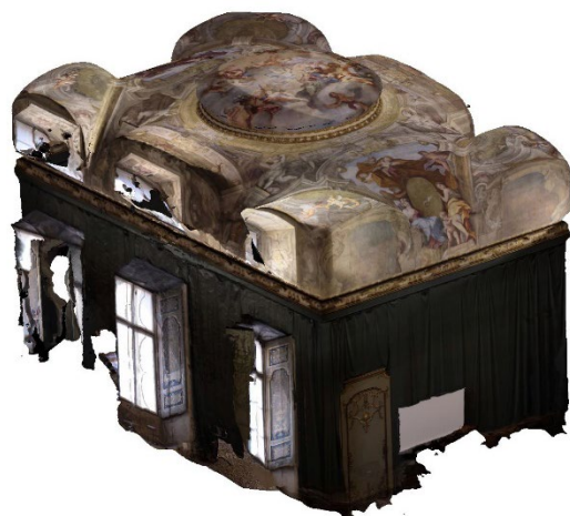
Figure 10. Textured mesh model from PhotoScan - 'Camera grande del letto' (Modelling: F. Natta)
