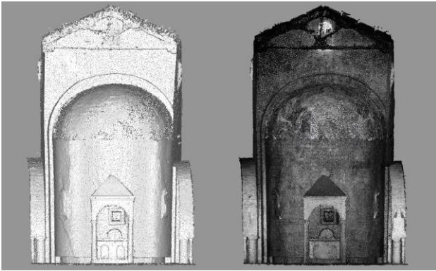
Figure 18. Hybrid point cloud generated from images of both Time 1 and Time 2.
