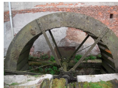
Figure 5. The overshoot water wheels of the Riviera mill: (a) Before the renovation (Courtesy of Arch. Roberto Olivero, 2004); (b) after the renovation.
