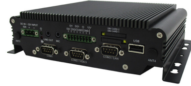
Fig. 2. Hardware for AGV from Navitech Systems [15]
