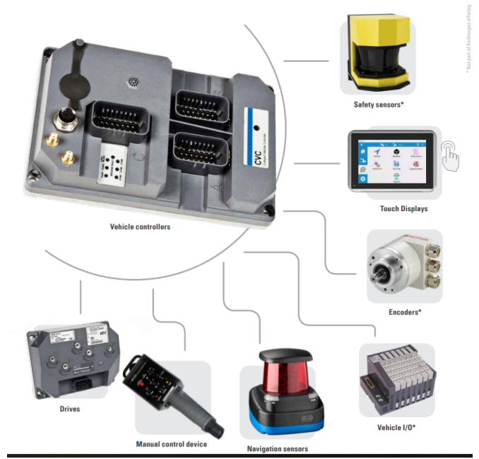
Fig. 1. Hardware ecosystem for AGV from Kollmorgen [14]
