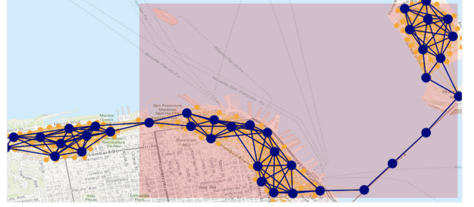
Figure 1: The reference topology we consider. Blue dots correspond to locations in \mathcal{L} , while orange ones correspond to zones in \mathcal{Z} . Blue lines connect locations between which UAVs can travel in one epoch; orange lines connect zones with the locations from which UAVs can provide coverage to them. The shadowed area corresponds to the small-scale topology we use for our comparison against the optimum.
