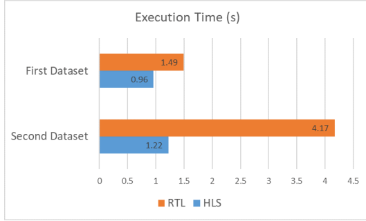
Fig. 5. Comparison of execution time for PCA algorithm between RTL [8] and HLS (this work).
