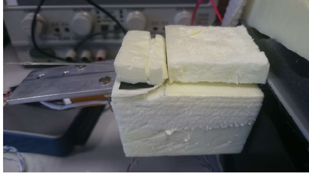
Figure 4.4: Picture of the setup during its use, where it is insulated to reduce heat dissipation.
