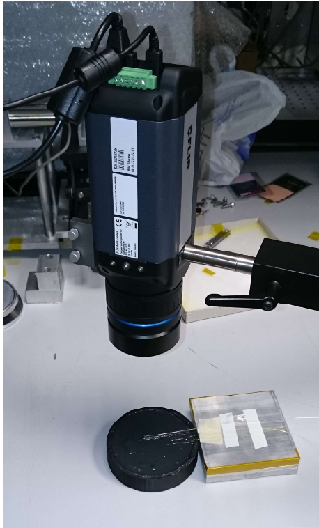
Figure 5.13: Position of the IR-Camera on the agar phantom to record the experiment temperature.
