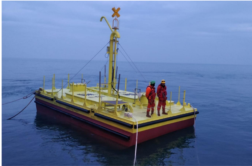
Figure 1.13 ISWEC 1:2 prototype deployed in Adriatic Sea off the coast of Ravenna (Italy), 2018.
