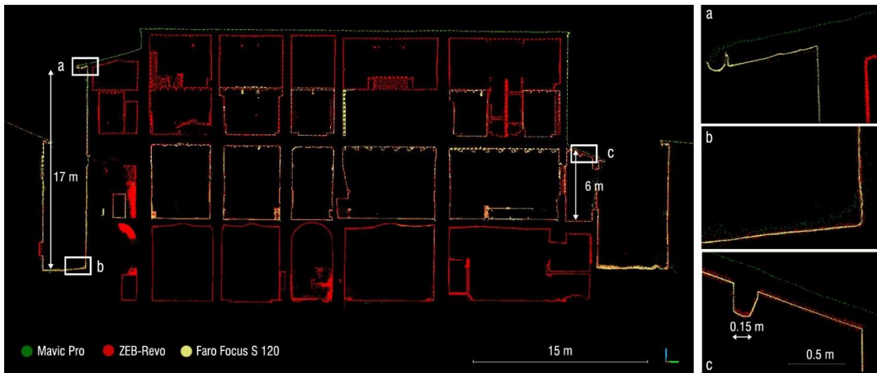
Figure 9. Longitudinal section of the point clouds with focus on three critical points: (a) upper part of the external façade, (b) corners, (c) elements in the ceiling.
