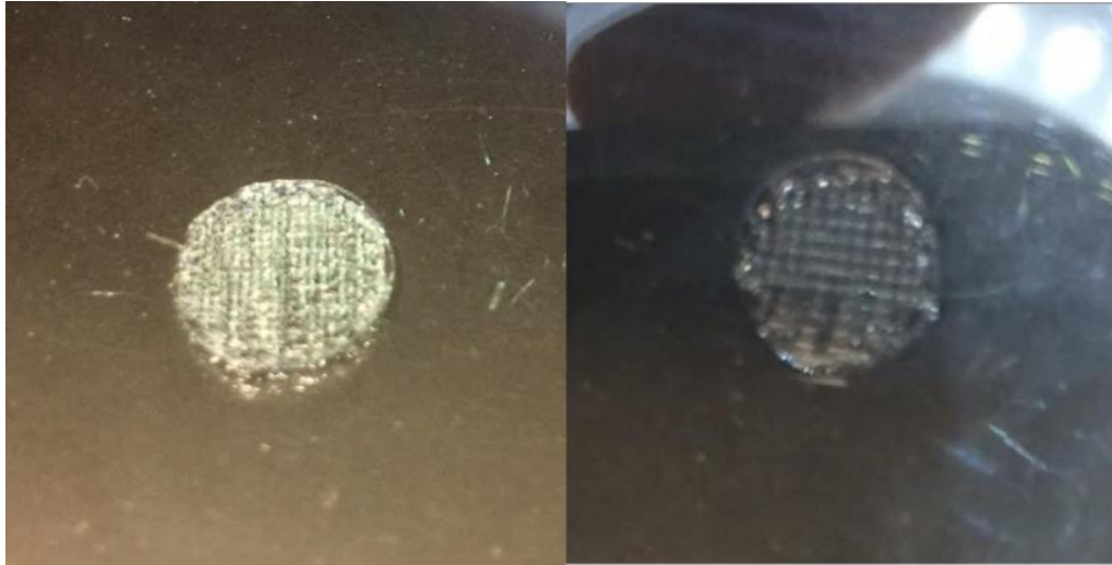
Figure 5.24 Pictures of the 3D printed circular scaffold (4 layers, grid pattern) obtained using the custom-made G-CODE and 210 and 450 \mu\text{m} nozzle diameter, respectively.
