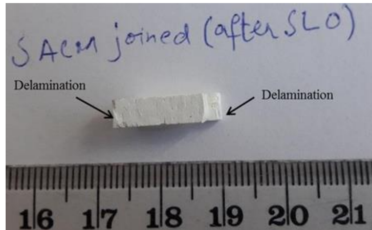
Figure 39: Delamination of the composite during SLO test
