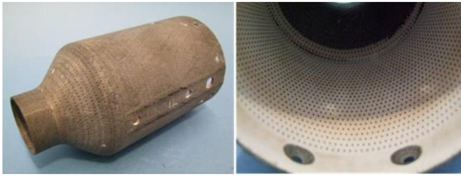
Figure 2: Condition of UMOX™ combustion chamber and EBC after testing (HiPOC)-Overall in good condition [15].
