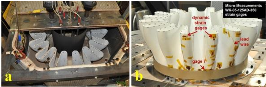
Figure 4: a) High temperature vibration testing and b) Vibration testing at Room Temperature [18]
