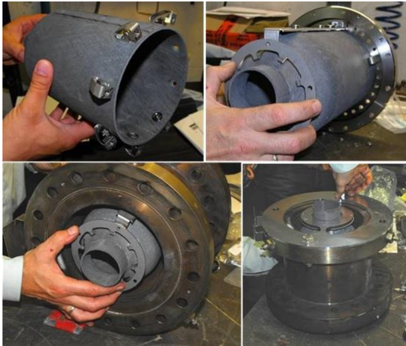
Figure 1: Successful fit check of UMOX™ combustion chamber (HiPOC) [15]
