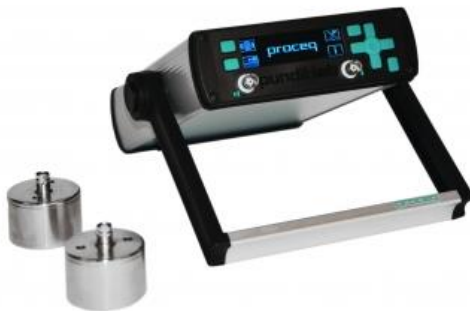
Fig. 4 – Particular of the sonotrode (a), built at this purpose by Sirius electrics, and of the generator/receiver (Pundit lab by Proceq from Pasi srl).
