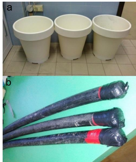
Figure 5. Materials used for laboratory test simulations: plastic cylindrical containers (a) and short segments of HDPE geothermal probes (b).
