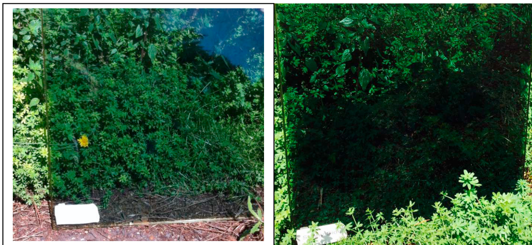
Fig. 1. Different states of TC glass, 400 x 400 mm sample under direct solar radiation.
