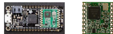
Fig. 2. Adafruit® Feather 32u4 LoRa Radio RFM9 on the left and LoRa Radio RFM9 transceiver module on the right.
