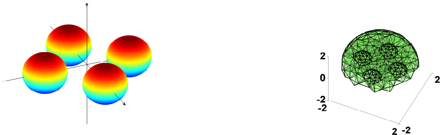
Figure 16: Example 4. The geometry of the problem: four spherical scatterers (left plot) and a section of the computational domain with a decomposition into tetrahedra (right plot).
