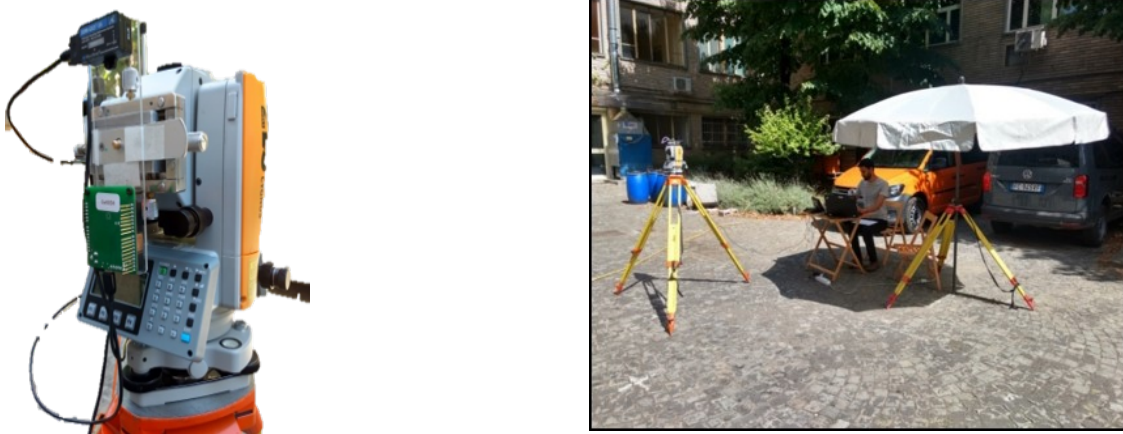
Figure 4.14: Inertial sensors fixed on a total station.
