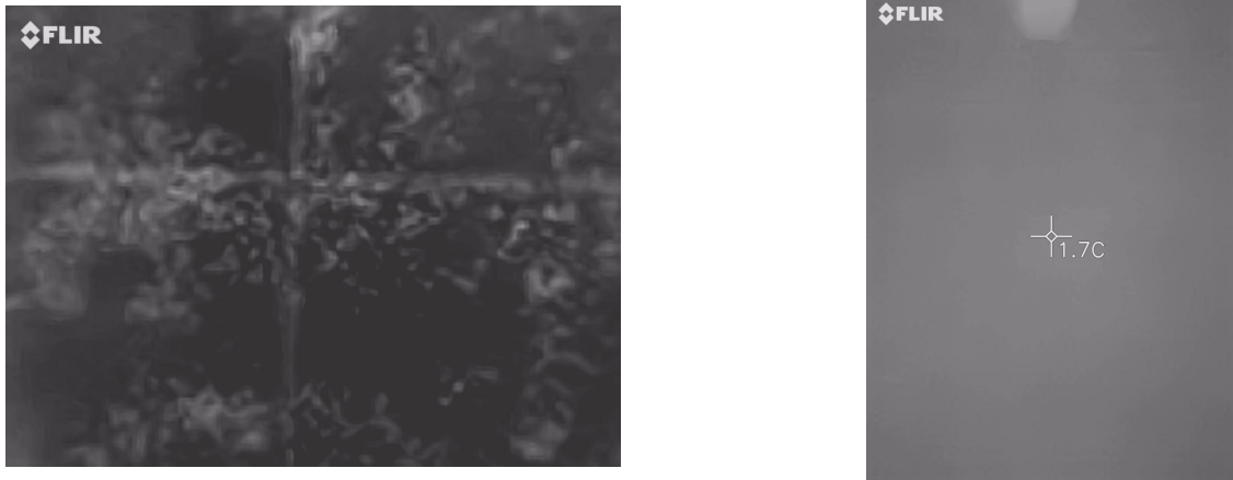
Figure 5.9: Comparison between thermal camera outdoor acquisition vs underground acquisition (Flir ONE Pro).
