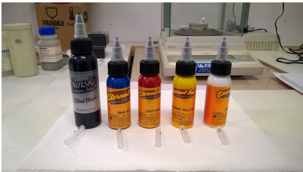
Figure 5.1: Five different commercial tattoo inks, involved in the electric and magnetic characterizations, just before being poured into the magnetic sample holders.
