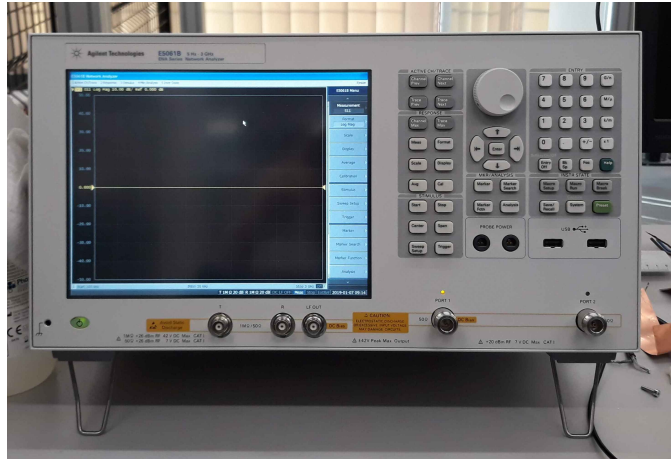
Figure 3.26: “Keysight E5061B ENA” employed in the birdcage coil impedance matching procedure.
