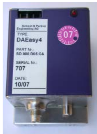
(b) Data Acquisition Electronics “DAE”.
