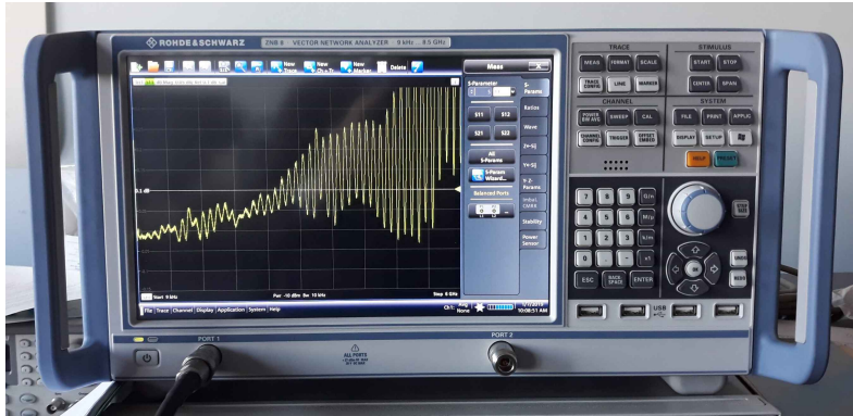
Figure 3.19: “Rohde Schwarz R&S ZND” Vector Network Analyzer used, together with the coupling loop, to measure the resonance frequencies of the birdcage coil.
