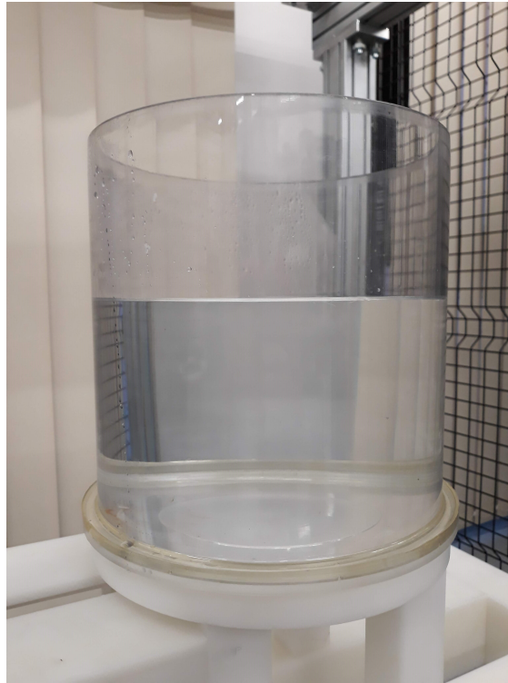
Figure 3.4: Cylindrical phantom employed in the experimental dosimetric set-up.
