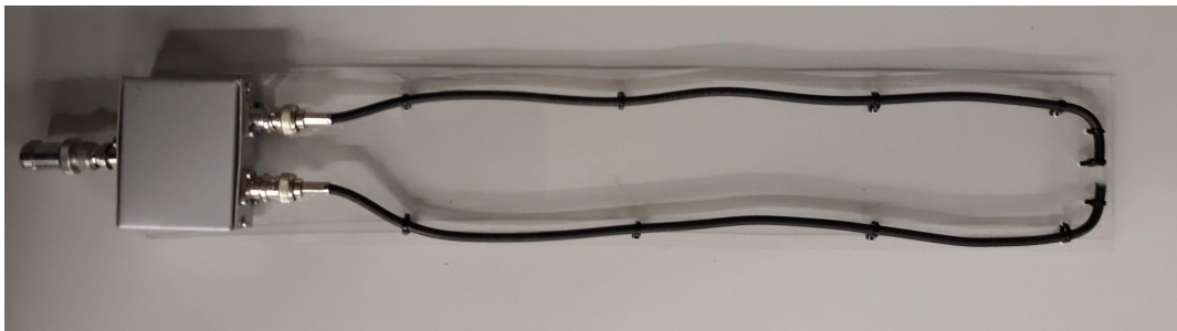
Figure 3.17: Picture of the shielded loop employed for the birdcage resonance frequencies measurement.
