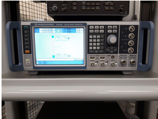
(a) “Rhode&Schwarz SMW200A” RF dual-channel vector signal generator.
