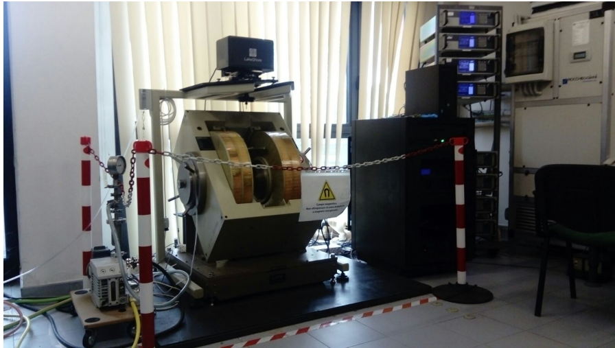
Figure 5.10: Lakeshore “7410 Vibrating Sample Magnetometer” employed for the magnetic measurements.
