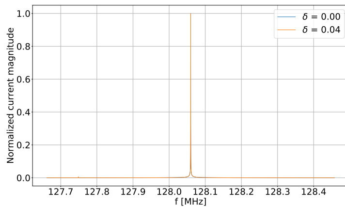
(b) Magnitude of the N/4 th mesh current due to a supply voltage applied to the same mesh.
