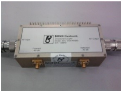
(c) “Bonn Elektronik DC 0125 40-250” bidirectional coupler.
