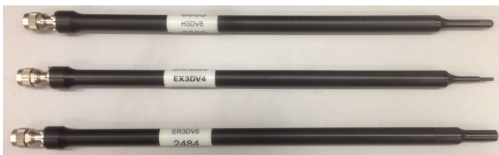
(c) RMS isotropic electromagnetic field probes. The above probe allows for magnetic field measurements both in air and inside the TSL. The bottom probe allows for electric field measurements in air whereas the middle one is specifically designed for electric field measurements inside the TSL.
