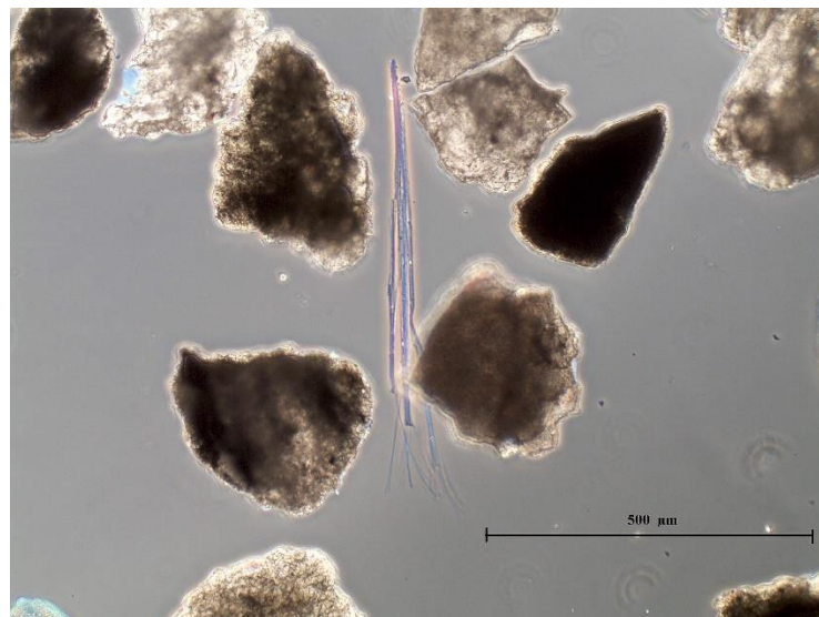
Figure 16: Chrysotile asbestos (refractive index oil n=1.550 )
