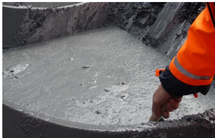
Figure 65: Sampling from the collection tank
