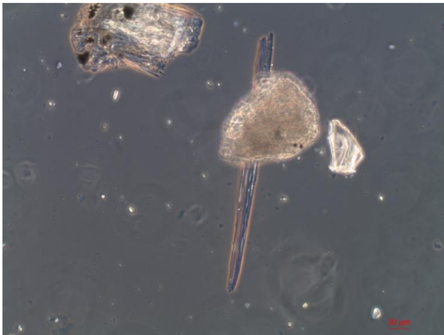
Figure 46: Antigorite refractive index oil 1.560
