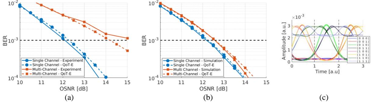
Figure 2. QoT-E vs experiment (a) and simulation (b) validation at  $D_{RES,IL} = 0$  ps/nm (a) and at  $D_{RES,IL} = 20$  ps/nm (b). Black dashed line sets the pre-FEC target BER. (c) ISI-distorted signal eye-diagram. Each color refers to one of the 8 patterns of  $M = 3$  bit.
