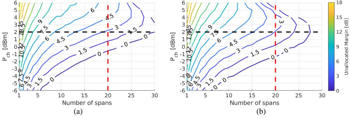
Figure 4. Unallocated Margin mask for (a) SMF network, (b) LEAF fiber network at  $\Delta f = 37.5$  GHz. Black dashed line is the  $P_{ch,max}$  constrained to EDFA total power of 22 dBm and 107 WDM channels. Red dashed line sets the maximum number of spans a path in the network. The color scale refers to both plots.
