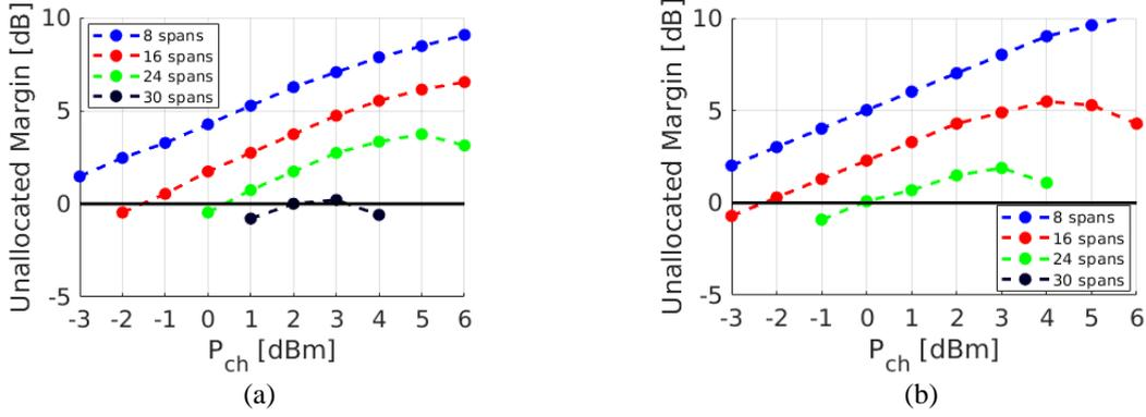
Figure 3. Unallocated Margin vs Channel power vs Number of spans for (a) SMF network, (b) LEAF fiber network at  $\Delta f = 37.5$  GHz. The black continuous line sets the zero-margin threshold below which the lightpath is out of service.
