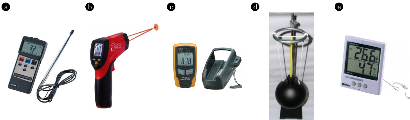
Fig. 3. Tools used in the experiment for monitoring, where: a) Photos of the TECPEL Hot Wire Anemometer to measure indoor air velocity b) CEM Dual Laser Infrared Thermometer to measure surface temperature from distance c) CEM USB Temperature and Humidity Data logger to measure indoor temperature and humidity d) Globe thermometer to measure globe temperature e) Tecpel thermo hygrometer to measure outdoor temperature by sensor.
