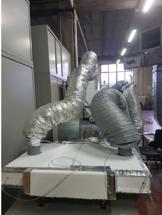
Figure 4. Adsorption heat exchanger
