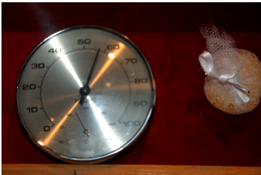
Figure 5.6: Thermo-hygrometer to measure T and RH in the museum and silica gel for reduce the RH inside the showcases
