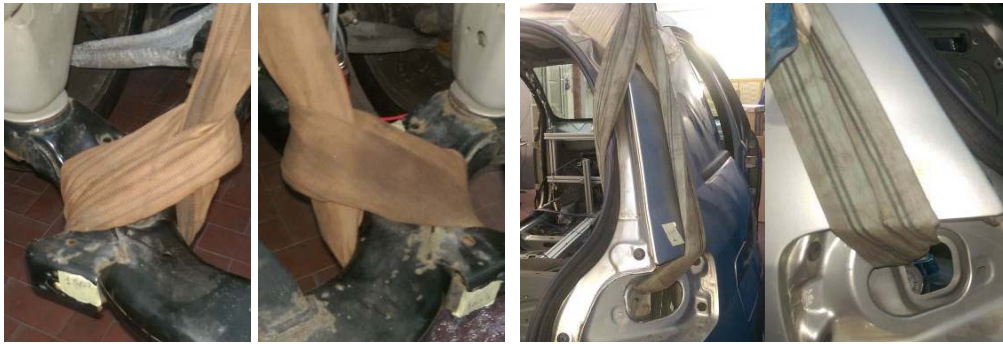
Figure 8.2 - Hanging points: front and rear, right and left (left to right).
