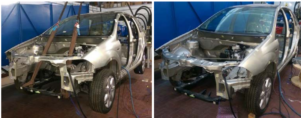
Figure 8.1 - Experimental setups configurations: MK (left) and MCK (right).
