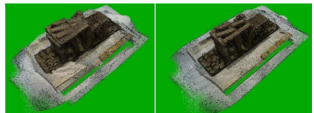
Figure 10. Point cloud after processing of the algorithm: online registration (left), HQ registration (right)
