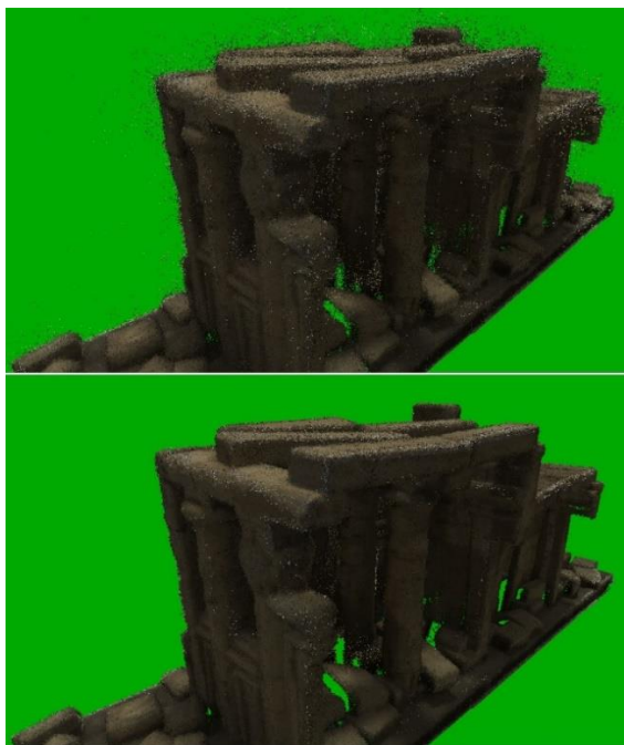
Figure 11. Point cloud before (top) and after (bottom) the SOR algorithm
