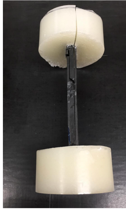
(b) Breakage of the resin support.
