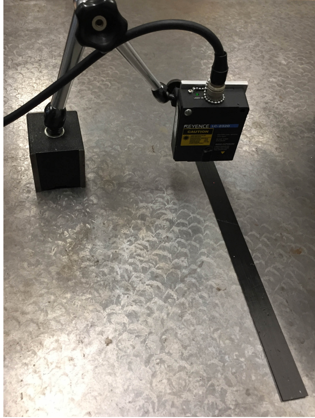
Figure 5.12: Geometric imperfection measurement of a monolithic beam.
