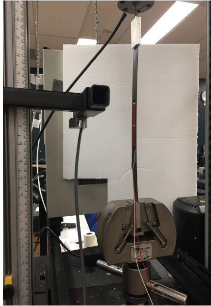
Figure 5.19: Experimental setup for the buckling test of beams with piezoelectric actuators.
