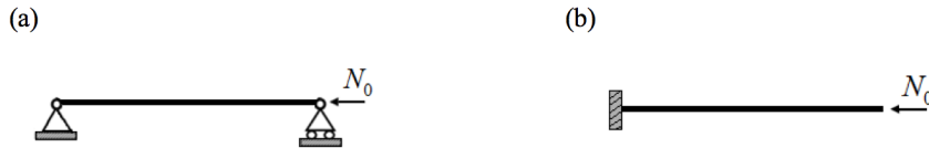
Figure 4.2: Load and boundary conditions: (a) simply-supported- (b) clamped-free-beam subjected to an axial-compressive force.
